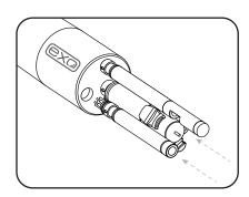
Do NOT leave any ports empty. Port plugs must be inserted into any port that does not have a sensor.
